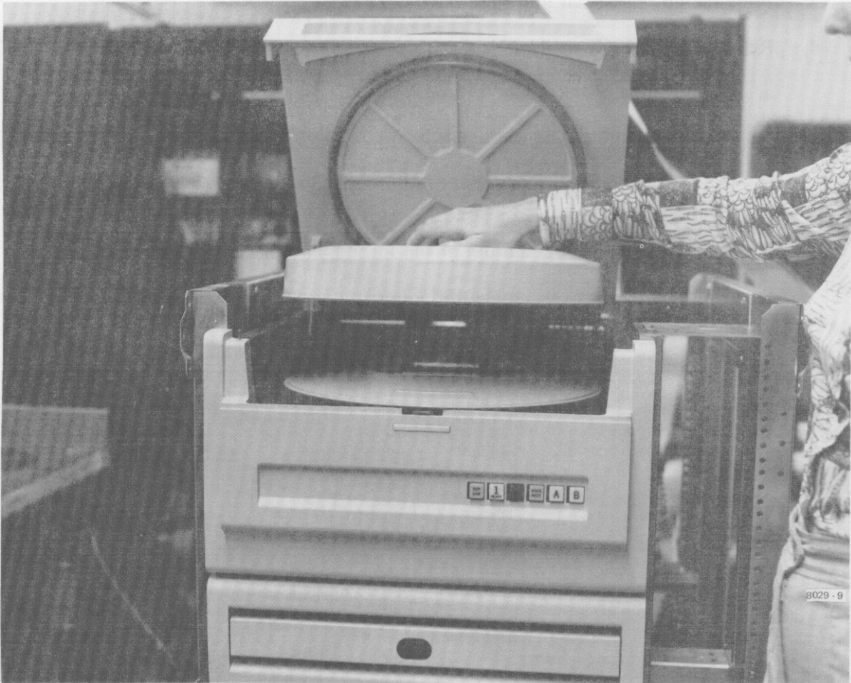
Figure 6-8 Installing Protection Cover
