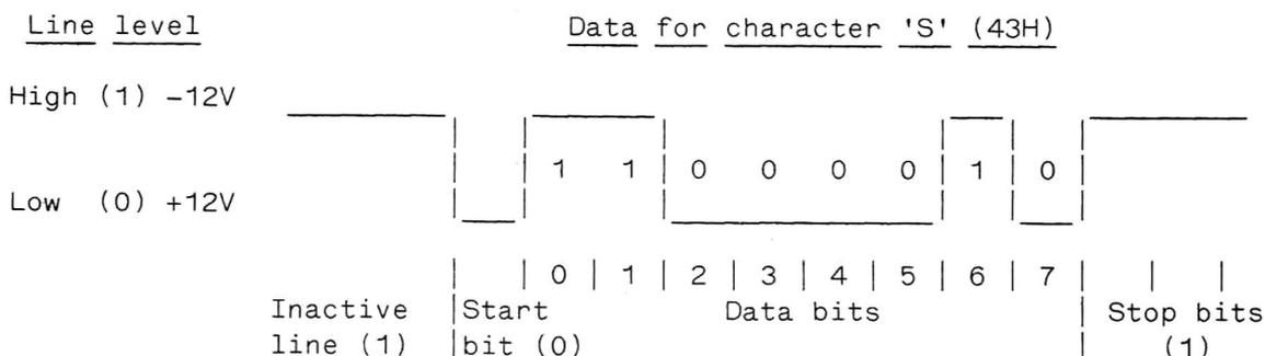
Each character sent over the serial data line is preceded by a start bit, which is always zero. This provides a synchronization point for the receiver. The data is then sent as 8 serial bits, with bit 0, the least significant bit, sent first. After the data, one or two stop bits are sent. These are at the same level as an inactive line, and are there to ensure some gap between characters.
