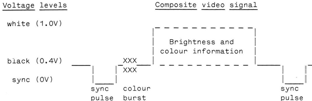
The sync pulses shown are for horizontal synchronization, and occur at 64us intervals. There are additionally vertical sync pulses which occur for about 0.5ms every 20ms.
