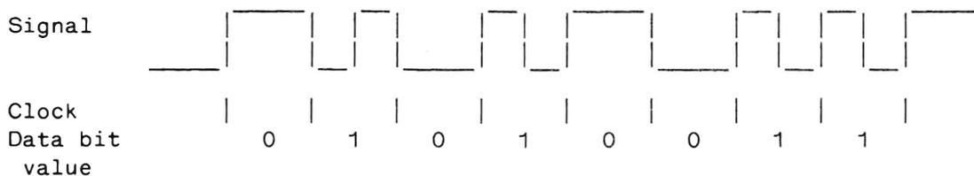
Data bytes are sent out on the tape end-to-end with no separating bits between them. There are three formats of tape; BASIC programs, SYSTEM tapes, and tapes holding data from PRINT#-1 statements. All tapes start with a leader, which is 256 bytes of zeros, followed by a sync byte which is 0A5H.
