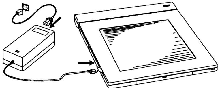
**Warning** Use only the ac/dc adapter supplied with your computer. Using a different adapter can damage the computer and/or the battery.
