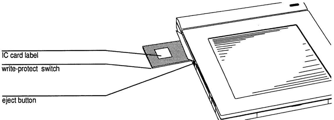
To remove an IC card, press the eject button. The IC card partially pops out.
