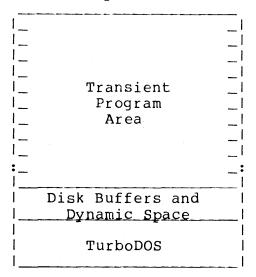
Since 8086-family processors can address up to a megabyte of memory directly, memory management is generally not a problem, and bank-switching is unnecessary.
