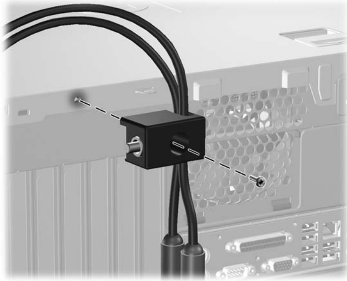
Figure C-5 Attaching the Lock to the Chassis
