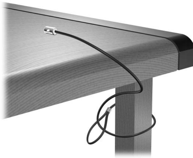
Figure C-3 Securing the Cable to a Fixed Object
