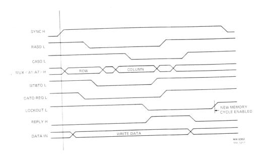
Figure A-2 DATO(B) Signal Sequence
