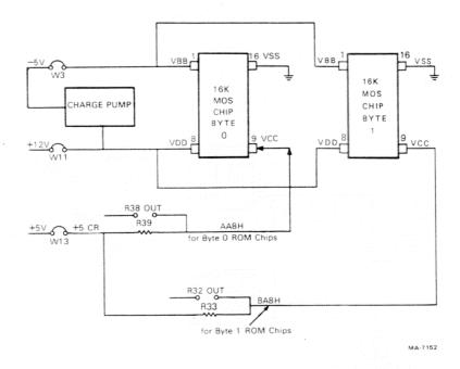
Figure 2-2 Triple Voltage MOS RAM without Battery Backup
