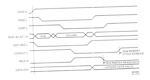
Figure A-3 DATI Signal Sequence
