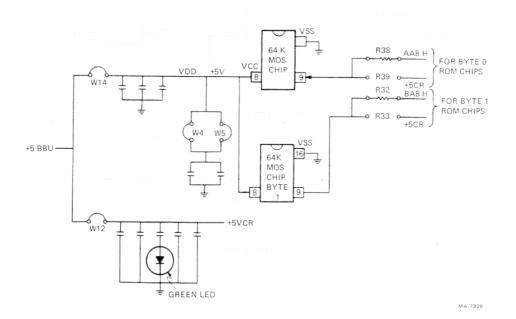
Figure 2-5 Single Voltage MOS RAM with Battery Backup
