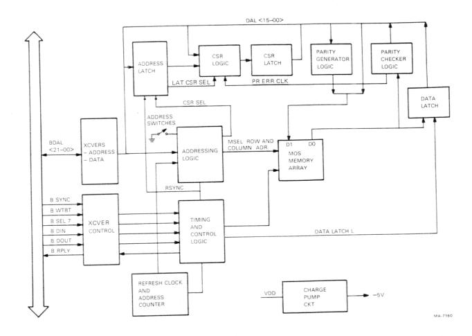
Figure 3-6 Logic Functions
