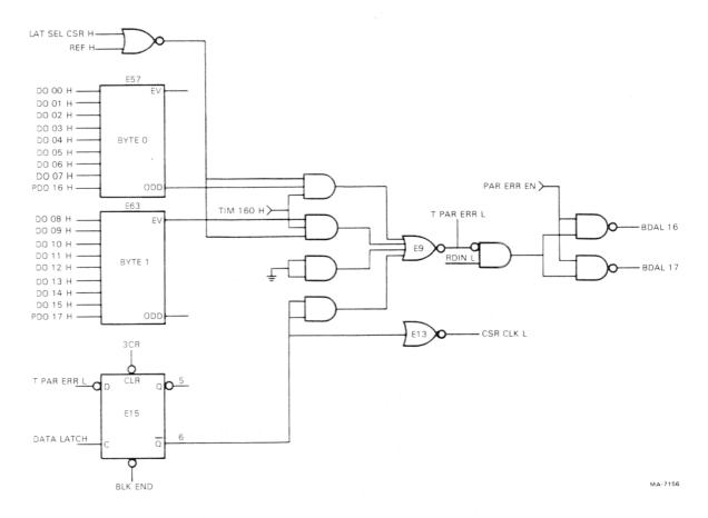
Figure 3-14 Parity Checkers
