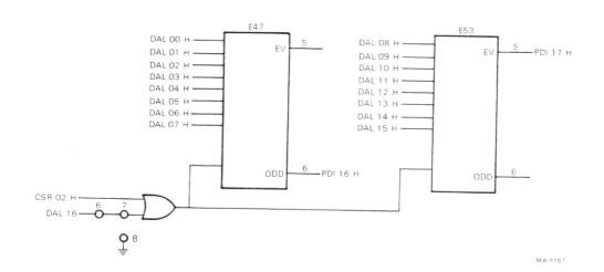
Figure 3-13 Parity Generators
