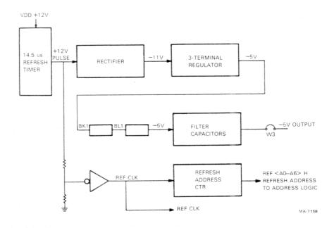
Figure 3-15 Refresh Logic and Charge Pump Circuit
