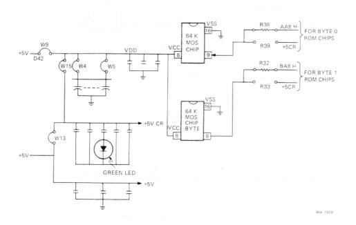
Figure 2-4 Single Voltage MOS RAM without Battery Backup
