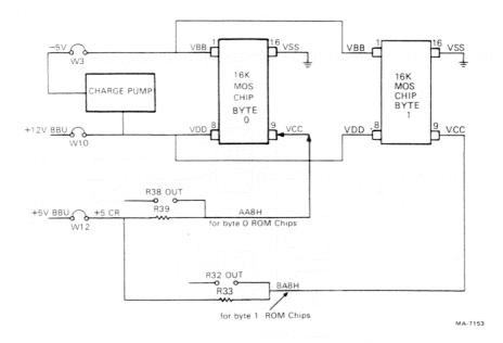
Figure 2-3 Triple Voltage MOS RAM with Battery Backup
