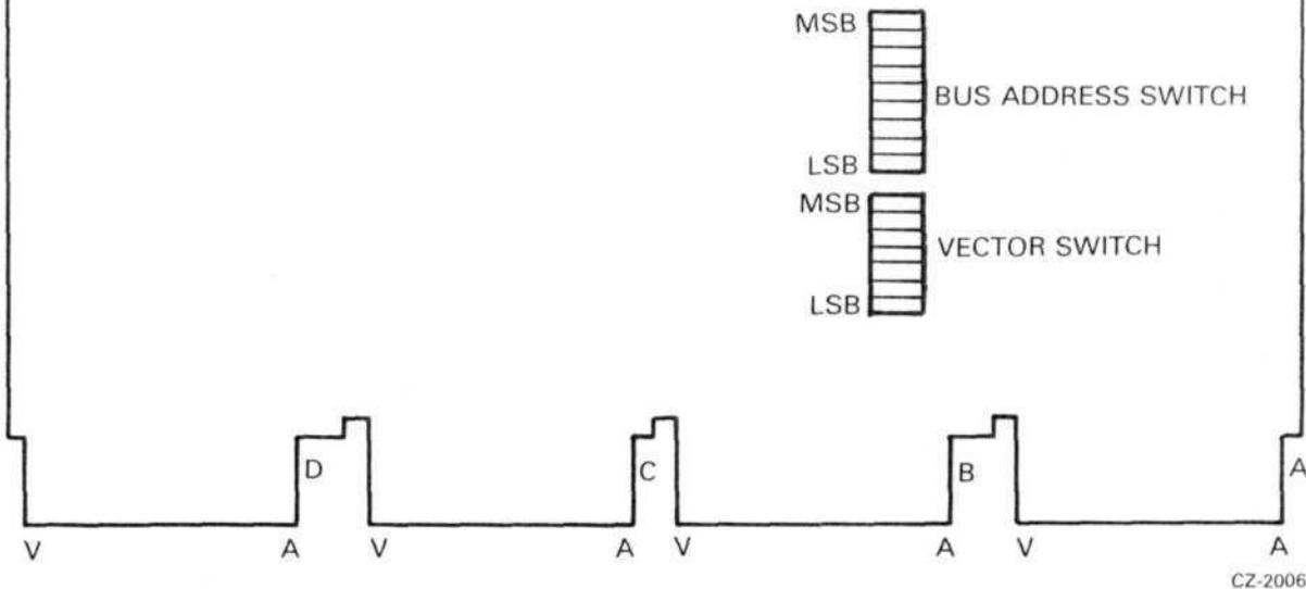
Figure 2-13 RLV11 Bus Interface Module (M8014) (Component Side)
