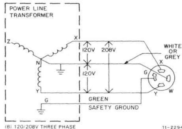
Figure 2-8 Three Phase Y Power System
