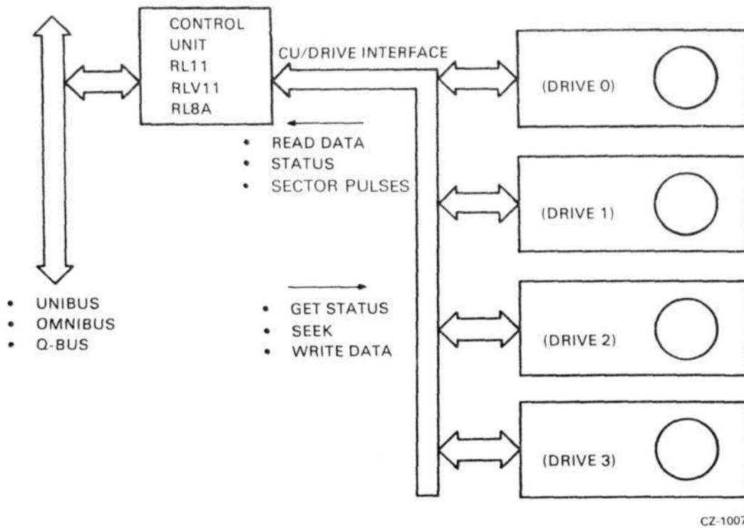
Figure 1-1 Typical RL01/RL02 Mass Storage Subsystem Configuration
