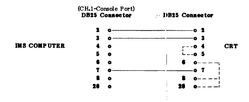
Note: Refer to the CRT manual to determine if it is necessary to tie pins 4 and 5 and pins 6, 8, and 20 together. This requirement will vary from one CRT manufacturer to another.
