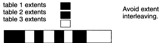
Figure 10-18 Illustration of interleaved extents
