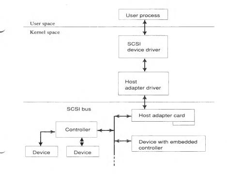
The SCSI kernel routines are contained in the development system software, and provide a vehicle for creating or maintaining SCSI device drivers and host adapter drivers. A *host adapter* is a card that converts computer-independent SCSI communications protocol to computer-specific information that your computer can process. A *SCSI bus* is a cable connecting a host adapter to a series of SCSI controllers and their associated devices.
