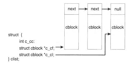
A protocol is defined for use with the *clists* to prevent a particular process or driver from consuming all available resources. Two constants for the *clist* high- and low-water marks are defined in the file named *sys/tty.h.* A process can issue write requests until the corresponding *clist* hits the high-water mark. The process is then suspended and I/O performed. When the list reaches the low-water mark, the process is awakened. Read requests use a similar protocol.
