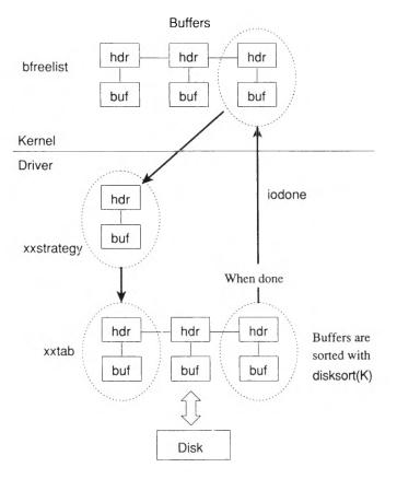
The driver validates the transfer parameters in the buffer header, and then queues the buffer on a doubly linked list of pending requests.
