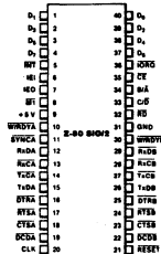
Figure 2. Z-80 SIO/2 Pin Assignments
